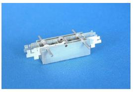
The two frames are inserted into the jig constructed earlier, where slots will accurately locate them. Axle steel can be inserted through the holes in jig and frames to lock everything in place. It may be necessary to slightly ream the axle bearings so that the rods will pass through, but this should be done very carefully so as not to excessively enlarge the holes. The frames can be inserted either way up into the jig, according to which way you find most
