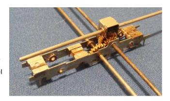
The wheels and stub axles are fitted in the usual manner – various articles in the 2mm Magazine and the Getting Started booklet cover this subject. Ensure that everything is turning freely at this stage. Remove the worm wheel stub axle in preparation for quartering and solder a crankpin into each wheel.
