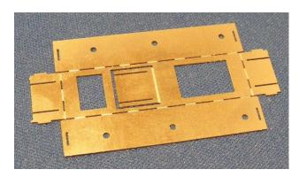
A special frame assembly jig is provided. It is recommended this is constructed now. It should be folded up and soldered. Check that the frame material will sit in the slots intended for them. Etching is not an exact science and however good a design, minor variations can occur in the etching process. It will be much easier to remove cusp at this stage rather than try to do it after the jig is constructed.
