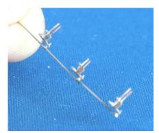
A small piece of balsa wood may be used into which the brass wire may be pressed through the chassis which is laid on its side to give a firm base on which to carry out the operation of fixing the brake rigging. Once this has been done the brake assembly can be withdrawn from the chassis and cleaned up. Using this method of assembly the brakes can be removed for maintenance.
