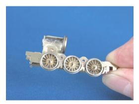
Solder the wire to the shoe assemblies and trim back that which is protruding on the front face of the shoes. Thread the longer lengths of wire through the etched holes in the side frames which, in conjunction with the shorter length brass wire, will correctly align the shoes in relation to the driving wheels.
