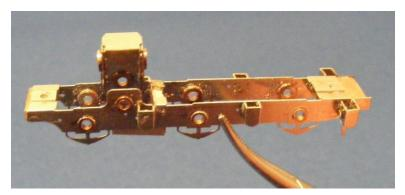
When all spacers have been fixed, the rods can be removed from the jig, and the chassis eased out. For certain locos etched sandboxes are provided, and these are most easily assembled and fitted at this stage. There may be locating holes etched into the chassis spacer tabs, these can now be used as templates to drill through the PCB spacers.
