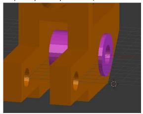
Ensure that the skew gear is a firm fit on the muff. Slide the gear into the slot at the bottom
