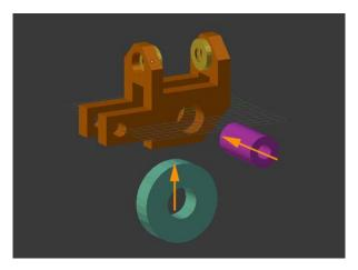
• Cut the worm to size. It should sit between the two frame bushes with the minimum of slop. Slide the worm between the bushes and insert either your motor shaft or the axle steel. The worm should rotate freely and in turn will now be meshed with the gear.
