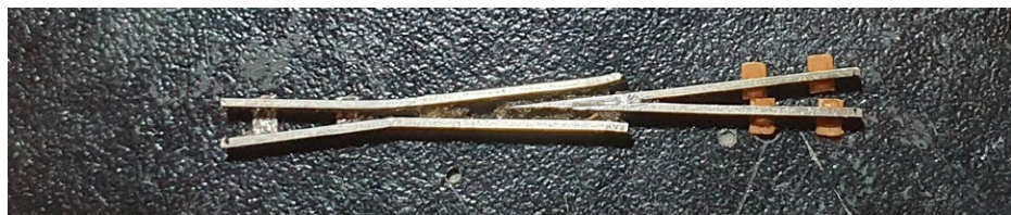
Figure 10. This is how I cut back the assemblies. The logic is that the four plastic chairs can be used to hold the assembly in place while the pads are soldered to copper clad sleepers. By the way, it is easier to thread the plastic chairs on before cutting back the rail – I found that out the hard way!
