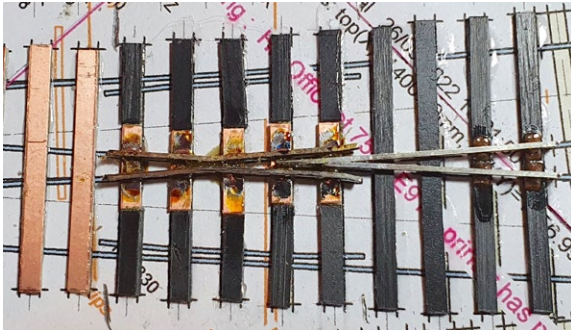
Figure 11. This should make more sense of Figure 10. You will note that I now no longer use full copper clad sleepers under the crossing nose as this arrangement allows me to use the Easitrac check rail chairs, which I find gives me a constant check rail/wing rail geometry. This picture shows the use of a crossing nose on a single slip.
