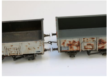
Figure 4. Shows the simple hook and loop coupling I have used on these wagons which gives very close coupling.
