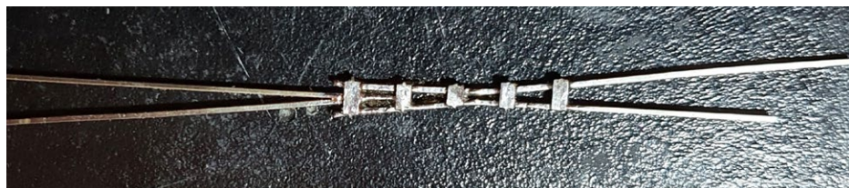
Figure 8. Completed assembly removed from jig – you can see the second stage soldering. Care should be taken here as the assembly can be tightly held and if you're not careful it can be damaged. At some point I suppose I could drill some release holes in the rail beds to allow pins to push out the assembly, but so far I have a 100% success rate at getting them out without damage.
