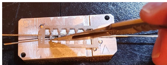
Figure 5. The etch is now placed on top of the rail, and once happy that it is located correctly it can be held in place with clips while soldering. I find a 3 mm tip on my 50W iron sufficient to sweat the pads in place. In a second stage of soldering, I apply a small amount of flux into the edge formed where the plates sit on the rail and apply a couple of solder balls. Because the solder paint has formed a connection between the rails and plates there is no heat sink issue. (Don't ask me why – there just isn't.) You could ignore this second stage, but I'd rather do the extra work than risk relying on the solder paint alone as the prospect of a crossing nose coming adrift when the points are in place doesn't bear thinking about!
