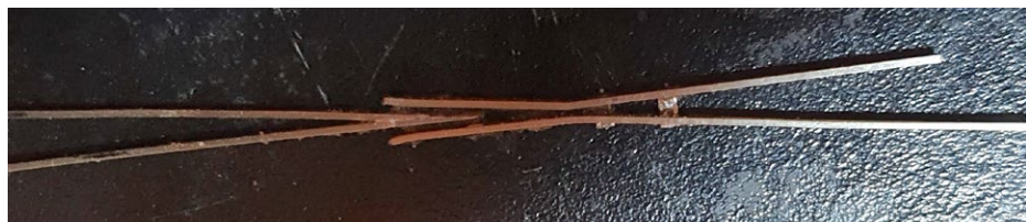
Figure 9. Completed assembly the right way up – all that needs to be done is cut the rails to length and lightly file back the bits of pad protruding out from under the rail.
