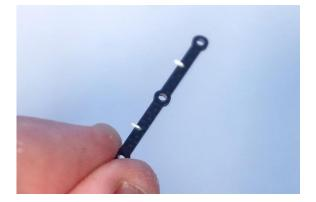
The pins can then be cut short leaving about 2 – 3mm of length as shown above.
