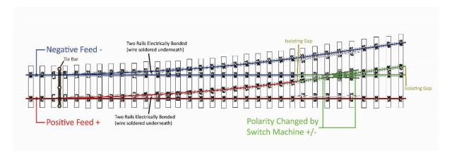
Each switch blade should be electrically bonded to its adjacent stock rail by soldering a small piece of wire between them under the rails at the point shown in the diagram.
