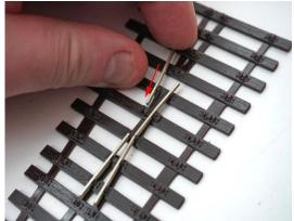
IMPORTANT! The join between the Wing Rails and the Closure Rails MUST be located exactly at the knuckle position. This position will be different for each kit, so you MUST refer to the downloadable template for your kit which will show the exact position of the knuckle. There is also a small indentation on the plastic base indicating the precise position of the knuckle join.
