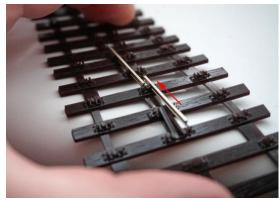
WARNING! – DO NOT over bend the plastic turnout base otherwise there is a risk of snapping the base! Only bend just enough to allow the rail to slide in.
