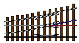
The Point rail is located on the main route and is inserted first and pushed all the way until it stops (it will wedge in). You should find the point of the V is 2 thirds over the sleeper.
