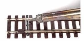
NOTE: Please only use a small amount of solder, otherwise there is a risk of solder flowing under the Switch Blade and bonding the Switch Blade to the Stock Rail.
