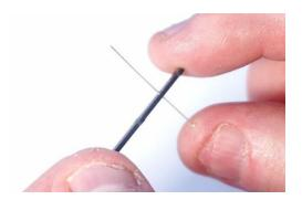
The 2 metal pins are inserted through the predrilled holes in the tie base.
