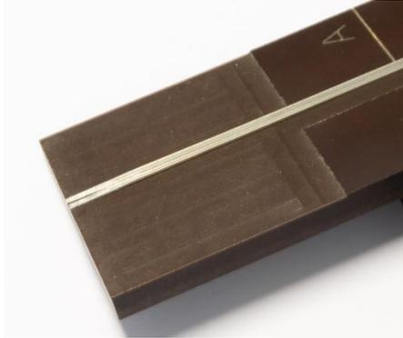
Work carefully until the abrasive stick is almost, but not quite, catching the end of the jig. At this point your switch blades will be correctly profiled.
