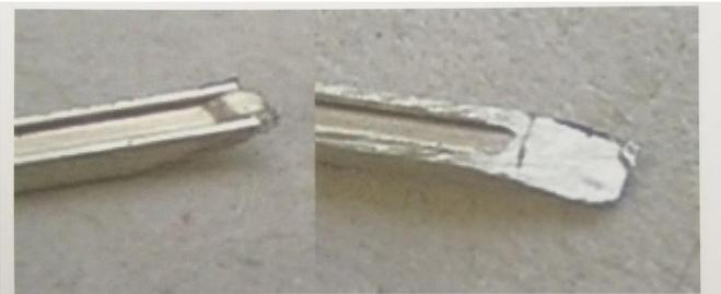
Fig 5.1 BH rail filed to a taper on one side only showing the wafer thin web. The presence of the very thin metal is just visible in the right hand picture as a pale area.
