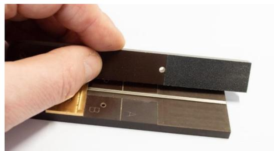
Only abrade the material on the outward stroke, not as the stick comes back, as there is a possibility of the abrasive catching on the rail ends.
