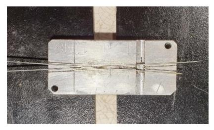
Crossing nose bits in jig ready for joining. The black line can be added to mark ends of the wing rails.
