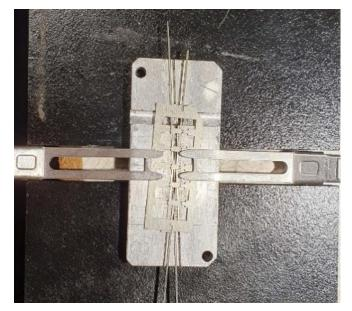
The etch positioned on the jig It is located using the slots and the folded under tabs. There's sufficient location to hold the etch in place but you may wish to add a couple of clamps. The best way to secure the etch to the rails is initially with solder paste which can then be reinforced, if required, with solder balls or solder wire. You will need a substantial iron to overcome the heatsink effect of the aluminium jig.
