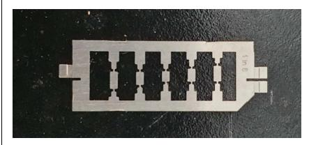
Etch ready for use. The half etches allow the little tabs to be folded under to act as location, making use of the fact that the top of the rail sits 5 thou above the jig.
