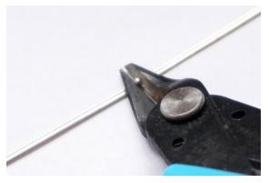
The small leg of metal that was connecting the Rail joiner to the Sprue needs to be cut off. This can be done using a pair of Side/Flush Cutters. Insert a second piece of scrap Bullhead Rail into the other side of the Rail Joiner and then lay this flat on its side on a suitable work area/table. Then use the Side/Flush Cutters to cut off the metal leg (WARNING: You MUST wear eye protection when doing this as the small leg of metal can easily ping off and into your eye).
