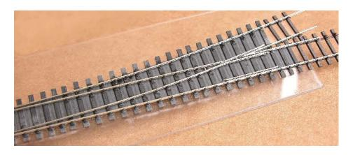
Above - Fig 19 shows the diverging stock rail has now been gauged in and fixed as has the point blade for the straight route. All that needs to be added is the checkrail for the diverging route.
