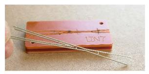
Left top - Fig 7 shows the crossing nose and the remainder of the common crossing rails in place in the jig. These rails will have small pieces of wire or old etch material depending on choice and availability soldered transversely across the rails to:-
