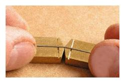
Above - Fig 6 shows the rail bending jig in use. It is probably best to very slightly over bend the angle and relieve it when inserting into the crossing assembly jig.
