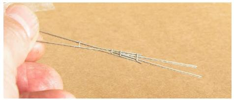
Above - Fig 10 is the common crossing assembly seen from beneath showing the soldered stretchers and the flange way rails cut back and bent using a pair of specially filed flat nosed pliers.
