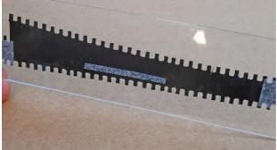
Left - Fig 2 shows the underside of the assembly where the method of securing the milled base to the sub-base by means of double sided adhesive tape can be seen. It was not felt necessary to use much more tape than is visible here for the aforementioned ease of removal
