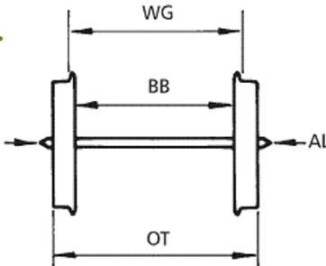
WG (wheel gauge) max. 9.12mm
