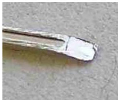
Figs 8 and 9 BH rail filed to a taper on one side only showing the wafer thin web. The presence of the very thin metal is just visible in the right hand picture as a pale area.
