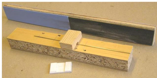
Fig 12 Filing board with wooden crossing block in position, styrene switch block in front and wet and dry file behind.
