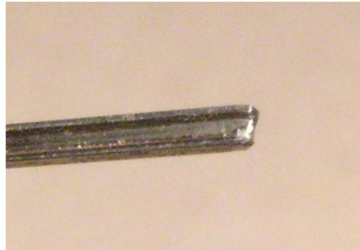
Fig 4 Rail end prepared for threading
