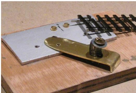
Fig 15 Heatsink for soldering wire connections to the bottom of the rail.
