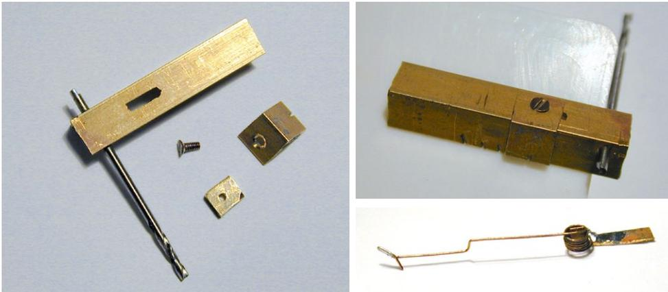
*The parts for adapting the winding jig (left), the adapted jig assembled (top right), and a resulting bogie coupling (bottom right).*
