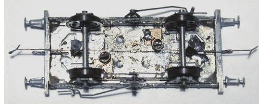
*The underside of an Association underframe with the two prototype couplings fitted. These were made from a 60mm length of 0.008" wire, as against the 30mm of 0.006" wire used for straight couplings. They are more flexible, but take up much less room than straight couplings, and can now be in line with one another resulting in a straight pull on the vehicle. They are also more robust and less prone to distortion.*
