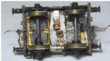
*This CR 8T swivel (single bolster) wagon illustrates just how short they can be made. This wagon is only 21mm over headstocks.*
