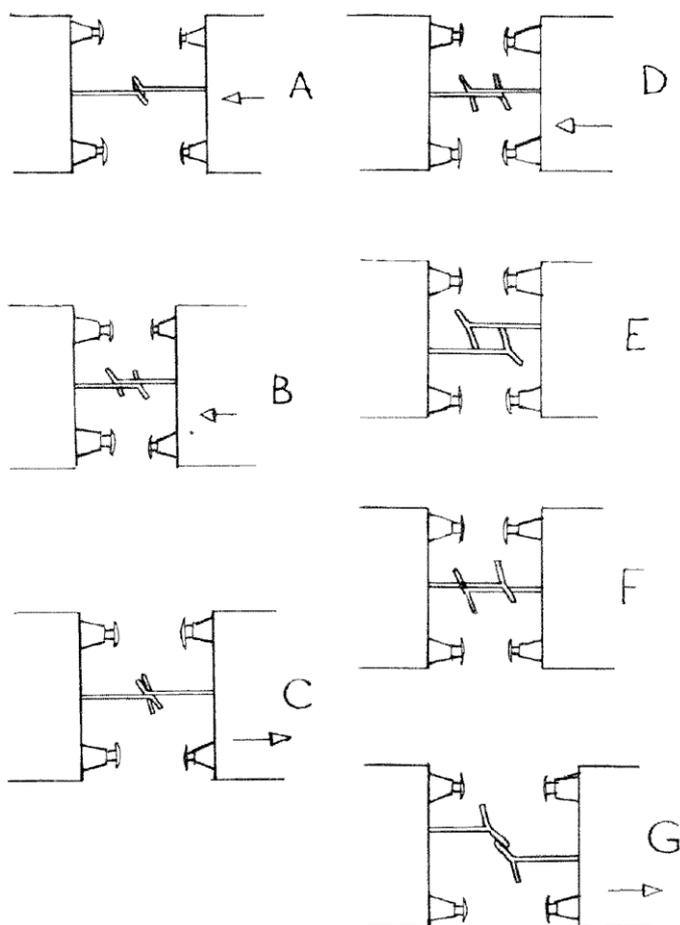
**Coupling:** on pushing two wagons together, the couplings move sideways (A) and spring past each other, springing back together (B), and on drawing away (C) the hooks lock together.
