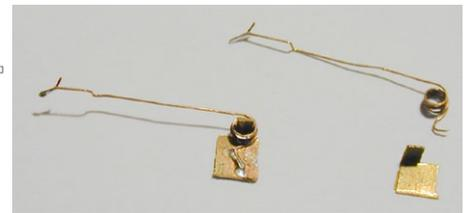
*Design for the coiled coupling, and two examples, one on its mount and the other with the mount beside it. (These were the prototypes and were wound the opposite way to the rest.)*
