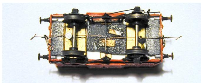
Even with such fine wire, straight couplings require such a length that, in most cases, they are attached to the underside of the vehicle beyond the transverse centre line. This results in them "passing" one another, as on this 9ft wheelbase wagon (15ft over headstocks). This is less than ideal as it results in a twisting force being applied to each vehicle in the train as they are pulled along.
