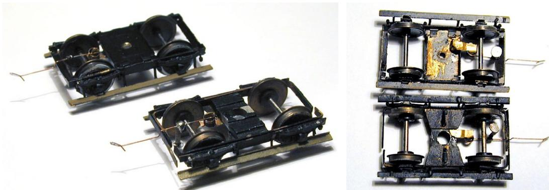
*Two different designs of bogie, from above and below respectively, with couplings fitted.*
